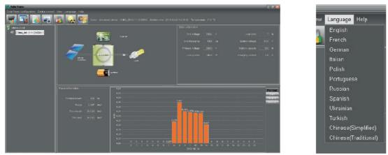
It comes with a multilingual extensive setup and monitoring software for reliable and transparent setup, as well as evaluation of your PV system. All the important operating parameters can be set via this program.
